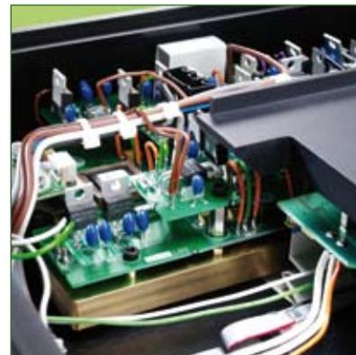
With clean signals of this sort the converter chip finds it easy to separate the control from the music signal. The latter is produced by an ultra-precise pulse generator directly in front of the converters. Naim has partitioned the quartz with triple regulated voltage and its own filters completely from the player electronics.
