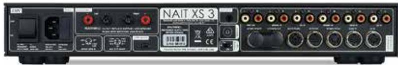
**ABOVE:** Crowded back panel includes USB upgrade socket, one set of 4mm speaker outputs and a preamp-out/power amp-in link. There's also a PSU upgrade input, variable line out, AV bypass, five line inputs (RCAs/DINs) and MM phono input (RCA)
