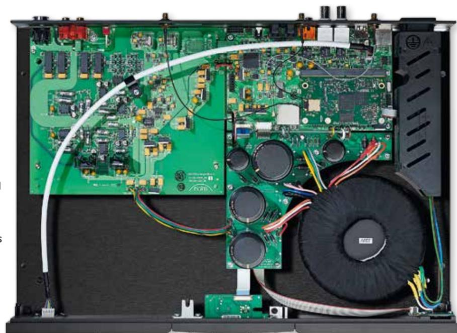
**RIGHT:** Substantial linear PSU [lower right] has independent regulation for Naim's custom streaming platform and FPGA-based filter/upsampling [top right PCB] and PCM1791 DAC-based analogue board [top left PCB]
