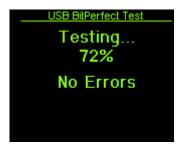
As the audio file progresses, the DAC-V1 will update the display to indicate how far through the test file it is, if any errors are found then they will be shown on this display.
