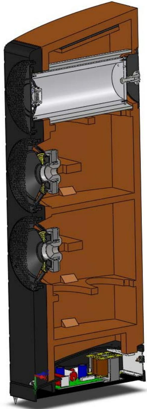
**Fig. 5** Speaker Cross-section
