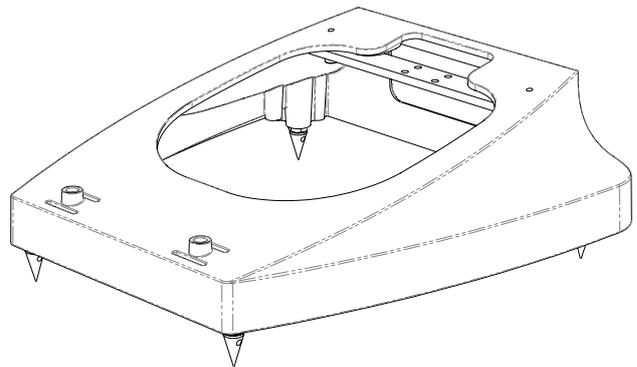
*A precision die-cast plinth houses the crossover module and incorporates a stainless steel leaf spring to decouple cabinet vibrations from the floor*
