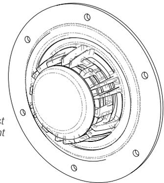
*Rear view of the Ovator BMR unit showing the die-cast chassis. An elastomeric mount decouples the BMR module from the main cabinet*
