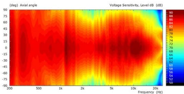
Directivity plot of a typical two-way system
