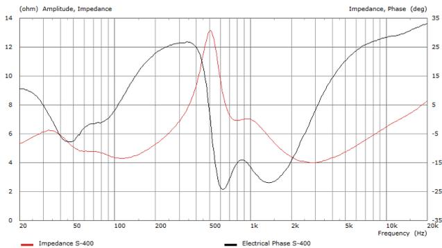
Impedance modulus (red trace) and phase (black trace) versus frequency
